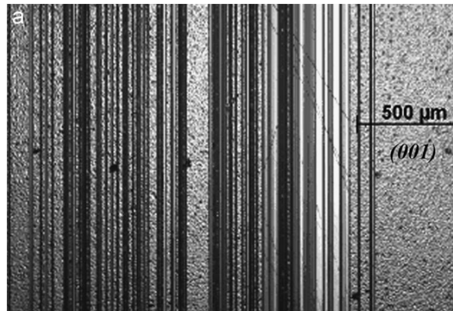
Etching pattern of a SBO sample. A. I. Zaitsev et al., J. Cryst. Growth 310, 1 (2008)
